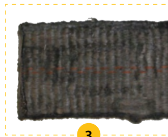
3 Excessive Abrasive Wear
