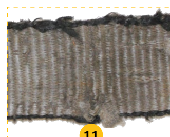
11 Excessive Abrasive Wear
